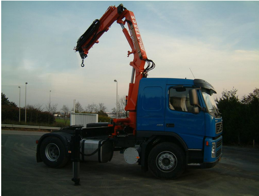
Image 6 AK 125CS A4: Another crane of the non-EU range. With 4 hydraulic extensions, the crane has an outreach of 12.3 meters (40'4") and a lifting capacity of 720 kg (1587 lbs) and is in the "medium crane range".
