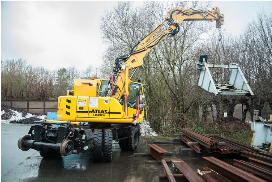
Image 3 1404 ZW: With an operating weight of 20,000 (44092 lbs) and powered by a 95 kW (130 hp) engine, the ATLAS rail-road excavator 1404 ZW is adaptable and flexible: the new computer-aided CARSY system ensures optimal contact pressure with the rails, which means highest traction capacity at lowest tire wear.
