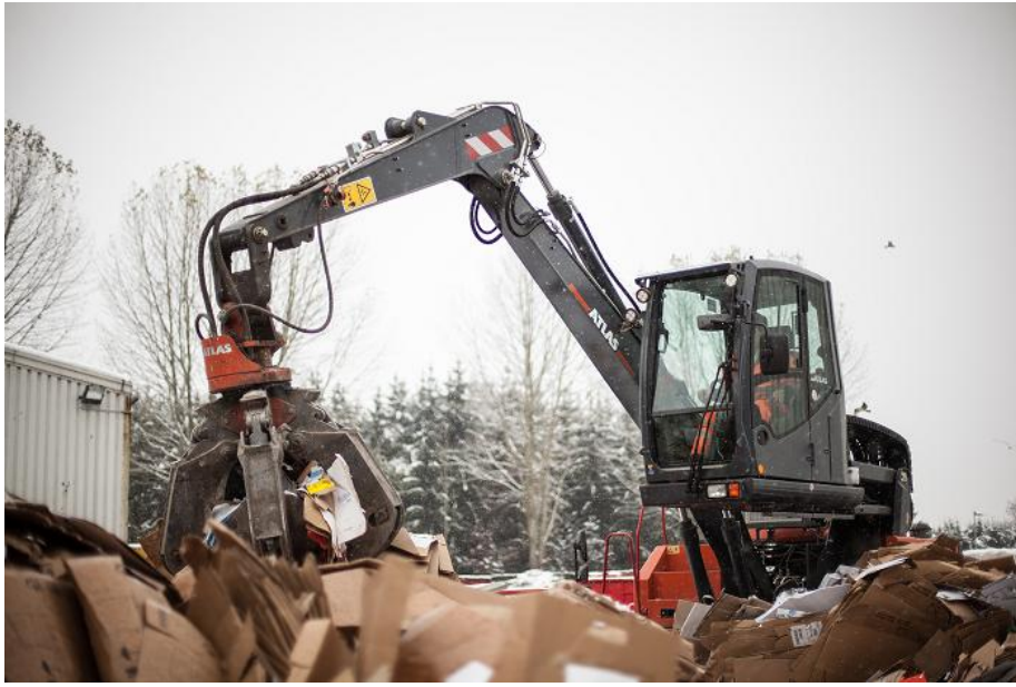
Image 1 160 MH: With a tail swing of less than 2 meters, the ATLAS material handler 160 MH belongs to the range of short-tail machines and is ideally suited for working indoors and in confined areas. Its average fuel consumption of less than 7 liters is also hard to beat.
