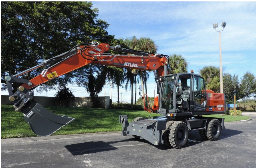
Image 4 190 W: Wheeled ATLAS excavators are the all-purpose excavators for road construction and civil engineering. Their enormous lifting capacity of more than 17 tons (37480 lbs), stability and mobility make it possible to work efficiently under almost any application conditions.
