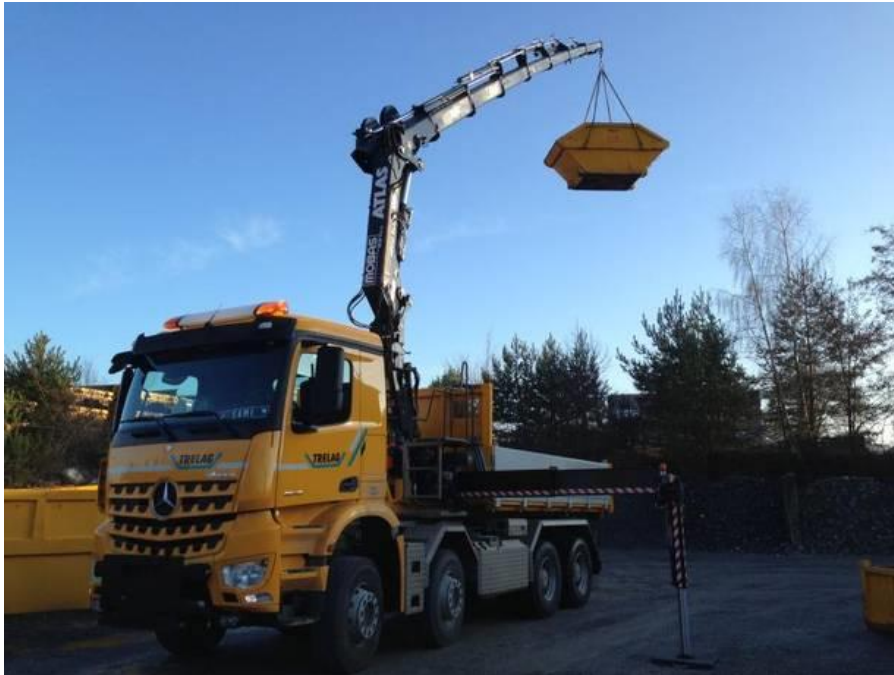
Image 8 AK 332.3 A8: And there is even a longer one: an impressive outreach of 21 meters (68'10") with 8 extensions, negative angle, and sensitive controls – the master of difficult tasks.
