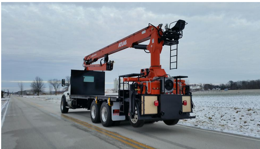
Image 9 AK 440 V CS: A great team: the Kenworth T-880 with an ATLAS loader crane type 440 V CS. The AK 440 V CS was specifically designed for the American/Canadian market and is mainly used for foundation engineering
